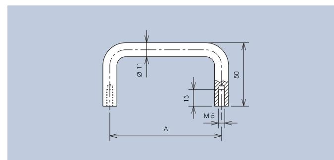
Offset bow-type handles for pulling, pushing and lifting actions for higher loads in mechanical, appliance and apparatus engineering.
