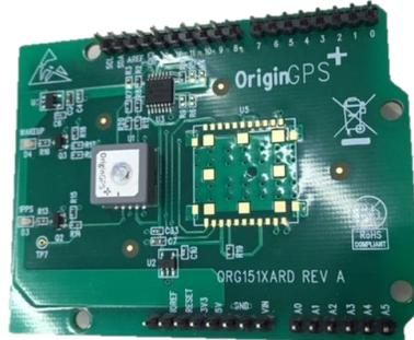
*The OriginGPS GNSS Shield for Arduino UNO Board*
