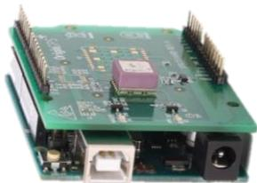
The OriginGPS shield is easily attached to the Arduino board by placing the shield on top of the board/s, and pressing gently till you hear a click. The OriginGPS GNSS shield enables you to navigate to your Arduino projects wherever they are.
