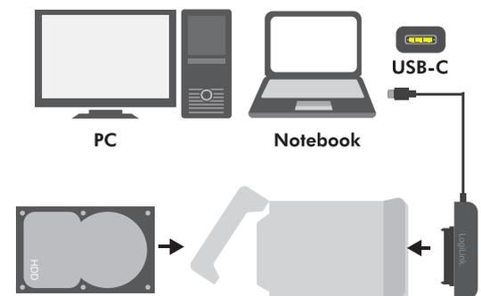
insert the HDD/SSD and connect to PC
