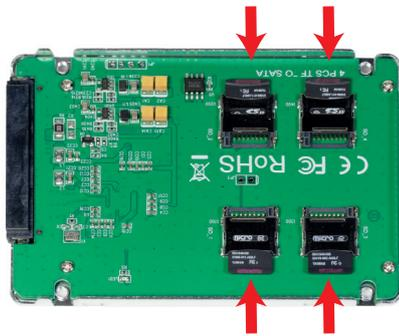
Insert 2 or 4 MicroSD cards into the MicroSD card slot.
