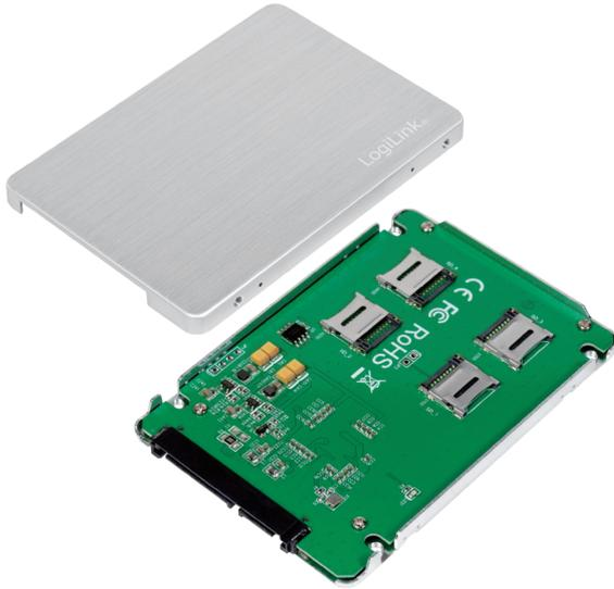
AD0022 is an economical choice to convert 4 MicroSD into a 2.5" SATA SSD storage device. Once being installed into PC/laptop, the 4 MicroSD appears as an ordinary SATA storage to any OS and can be configured as a boot disk.
