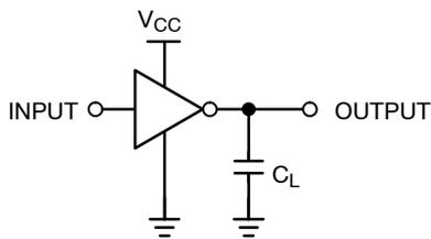
C<sub>L</sub> includes load and stray capacitance
