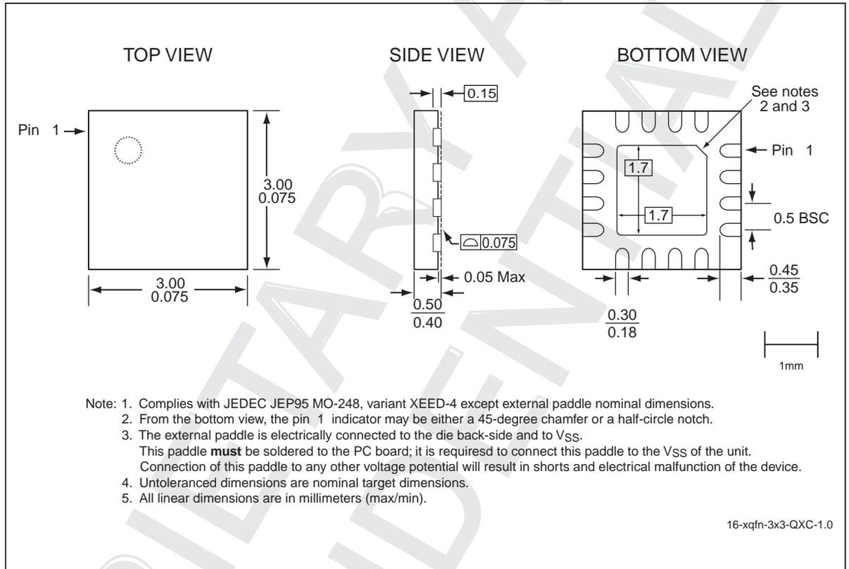
**Figure 10:**16-contact Extremely-thin Quad Flat No-lead (XQFN)
