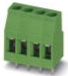
PCB terminal block, nominal current: 24 A, nom. voltage: 400 V, pitch: 5.08 mm, number of positions: 8, connection method: Screw connection with tension sleeve, mounting: Wave soldering, conductor/PCB connection direction: 0 °, color: green. The article can be aligned to create different nos. of positions!
