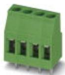
PCB terminal block, nominal current: 24 A, nom. voltage: 400 V, pitch: 5.08 mm, number of positions: 4, connection method: Screw connection with tension sleeve, mounting: Wave soldering, conductor/PCB connection direction: 0 °, color: green. The article can be aligned to create different nos. of positions!
