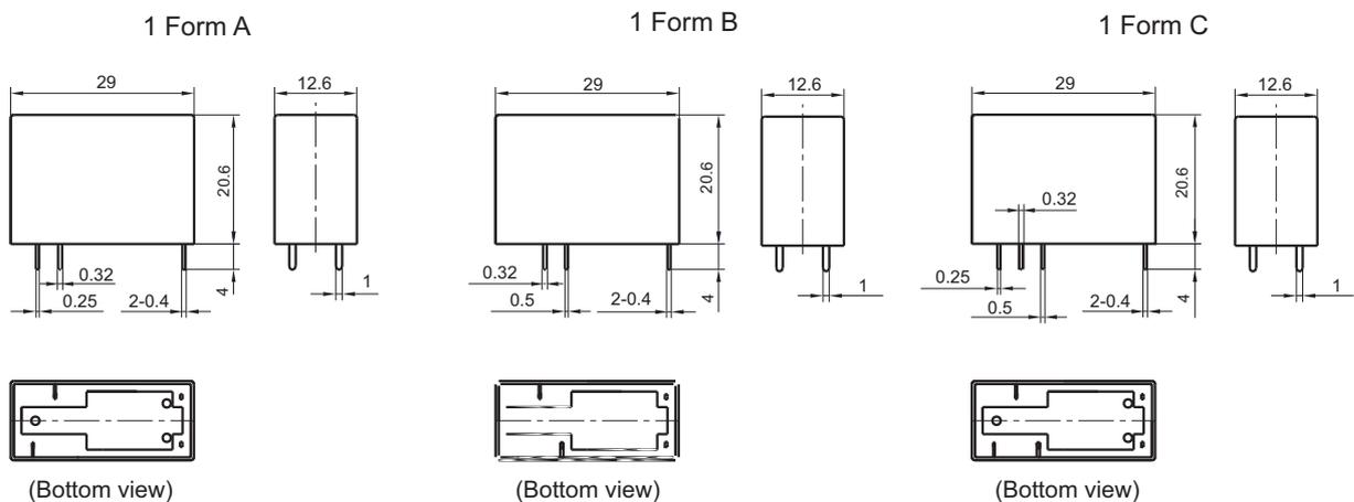
Remark: 1) In case of no tolerance shown in outline dimension: outline dimension  $\leq 1\text{mm}$ , tolerance should be  $\pm 0.2\text{mm}$ ; outline dimension  $> 1\text{mm}$  and  $\leq 5\text{mm}$ , tolerance should be  $\pm 0.3\text{mm}$ ; outline dimension  $> 5\text{mm}$ , tolerance should be  $\pm 0.4\text{mm}$ .
