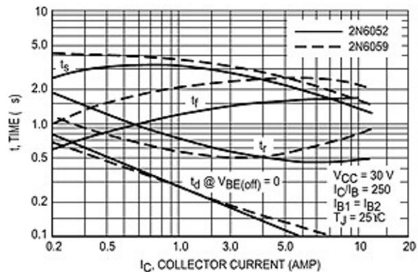
Figure 3. Switching Times
