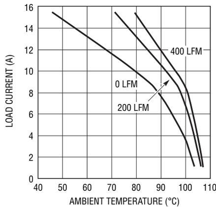
**Figure 12. 5V<sub>IN</sub> to 1.2V<sub>OUT</sub> with BGA Heat Sink**
