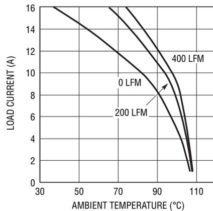
**Figure 16. 3.3V<sub>IN</sub> 2.5V<sub>OUT</sub> with BGA Heat Sink**
