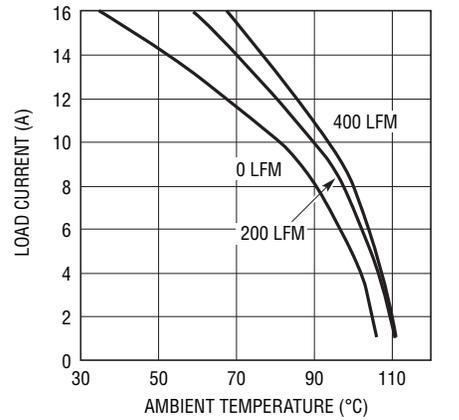
**Figure 14. 3.3V<sub>IN</sub> to 2.5V<sub>OUT</sub> with No Heat Sink**
