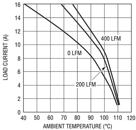
**Figure 15. 3.3V<sub>IN</sub> 1.2V<sub>OUT</sub> with BGA Heat Sink**
