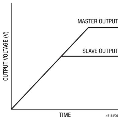
Figure 6. Output Voltage Coincident Tracking
