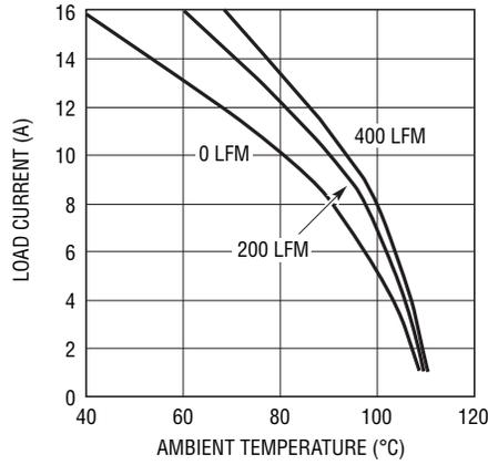
**Figure 13. 3.3V<sub>IN</sub> to 1.2V<sub>OUT</sub> with No Heat Sink**
