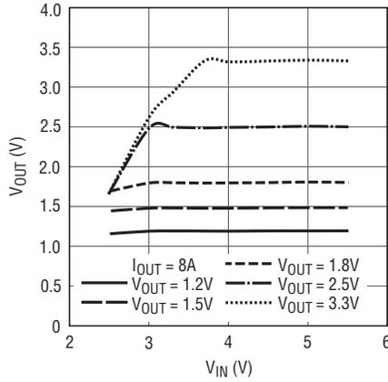
**V<sub>IN</sub> to V<sub>OUT</sub> Step-Down Ratio**
