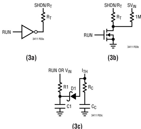
Figure 3. SHDN/R<sub>T</sub> Pin Interfacing and External Soft-Start
