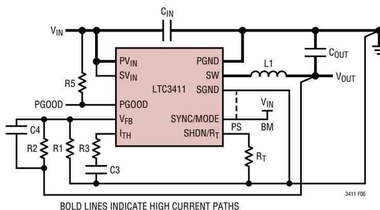
Figure 6. LTC3411 Layout Diagram (See Board Layout Checklist)
