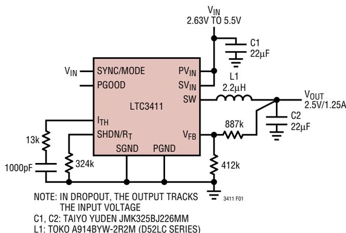
Figure 1. Step-Down 2.5V/1.25A Regulator
