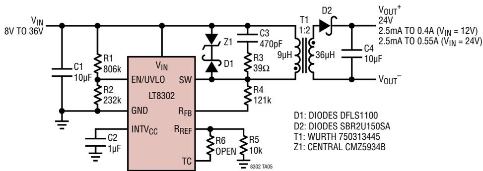
8V to 36V<sub>IN</sub>/48V<sub>OUT</sub> Isolated Flyback Converter
