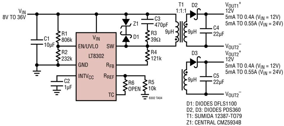
8V to 36V<sub>IN</sub>/24V<sub>OUT</sub> Isolated Flyback Converter
