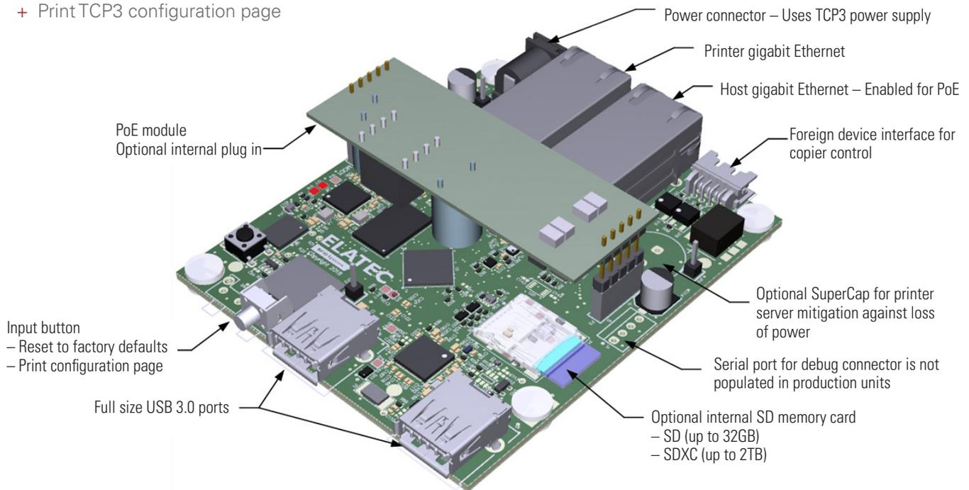
From secure printing to industrial robotics, TCP3 enables user authentication and access control security for devices that lack a USB port.
