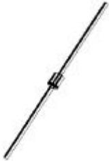
Polarity: Cathode is marked by band
